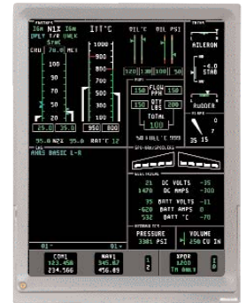
EICAS - Engine Information, Aircraft Systems, Crew Messaging and Radio Tuning
